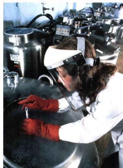
Fig. 3. One method of preserving cultures at ATCC is storage in liquid nitrogen. This technician is removing a canister containing culture vials from a vat of liquid nitrogen.
