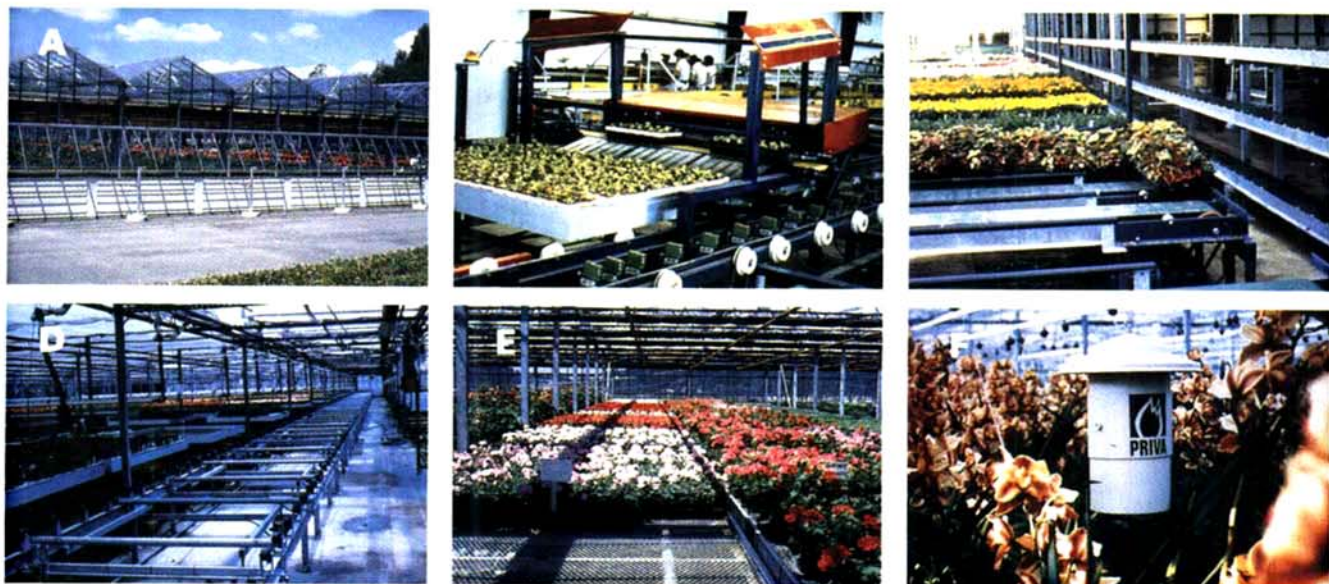
Fig. 9. Mechanized systems for improved crop management in greenhouses will be a major thrust during the next decade. (A) Modern facilities include (B) automated potting and loading equipment, (C) conveyor systems, (D and E) movable benches, and (F) computer-controlled environmental conditions. (Figs. B, C, D, and F courtesy V & V Noordland, Inc.)
