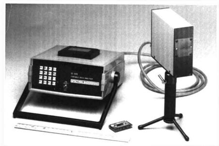
photometer, computer-controlled programmable motorized precision stepping stage, and software package.
