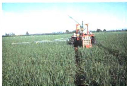
Fig. 4. Spray rig used for applying fungicides from the edge of a treatment plot.
