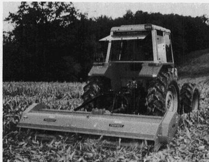
The rotor is connected to the tractor's P.T.O. by a flexible indirect drive. The KV-320 features a full-length rear roller with skids at both sides for easy handling on all types of terrain.
