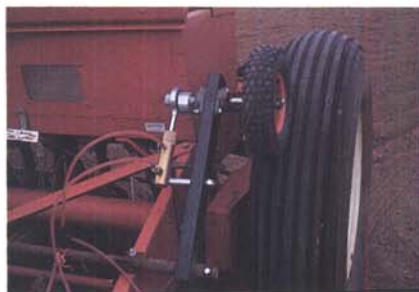
Fig. 9. Acrameter pump for applying EDB mounted on a seeder.
