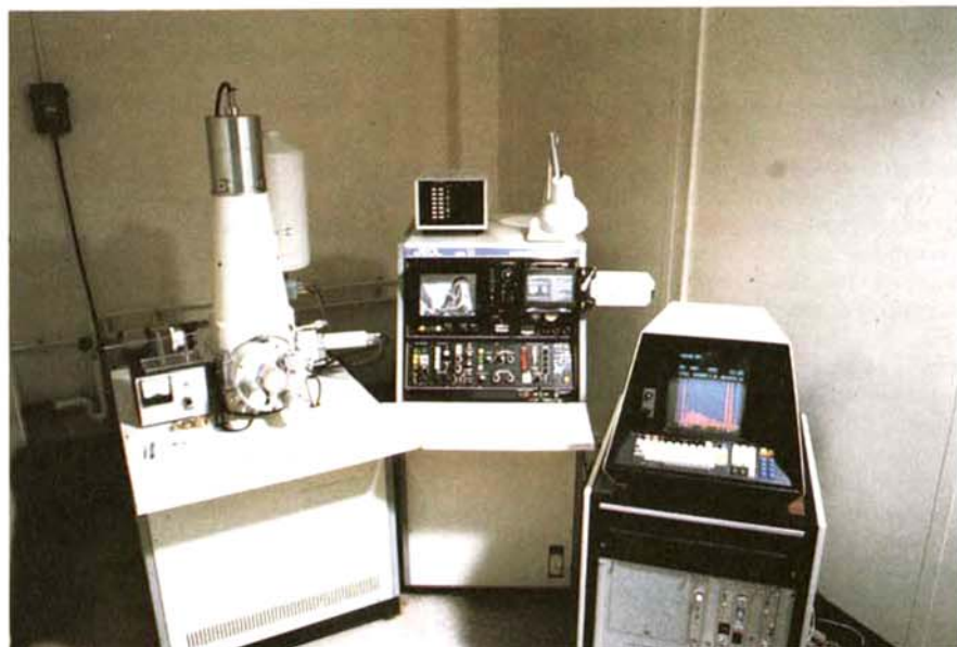
Fig. 1. A high-resolution scanning electron microscope equipped with an energy dispersive X-ray analyzer.
