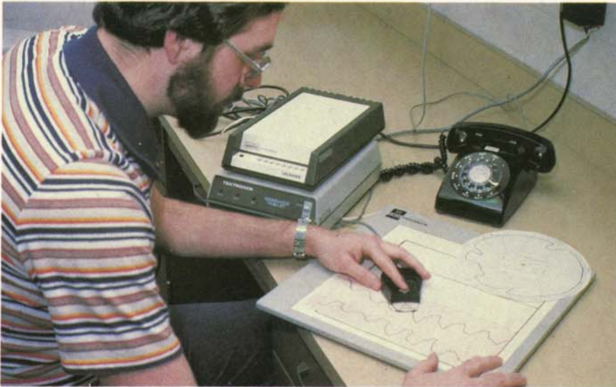
Fig. 6. Use of a digitizer to transcribe environmental data from strip charts.
