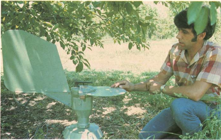
Fig. 5. Collection of ascospores with a Burkard volumetric spore trap.
