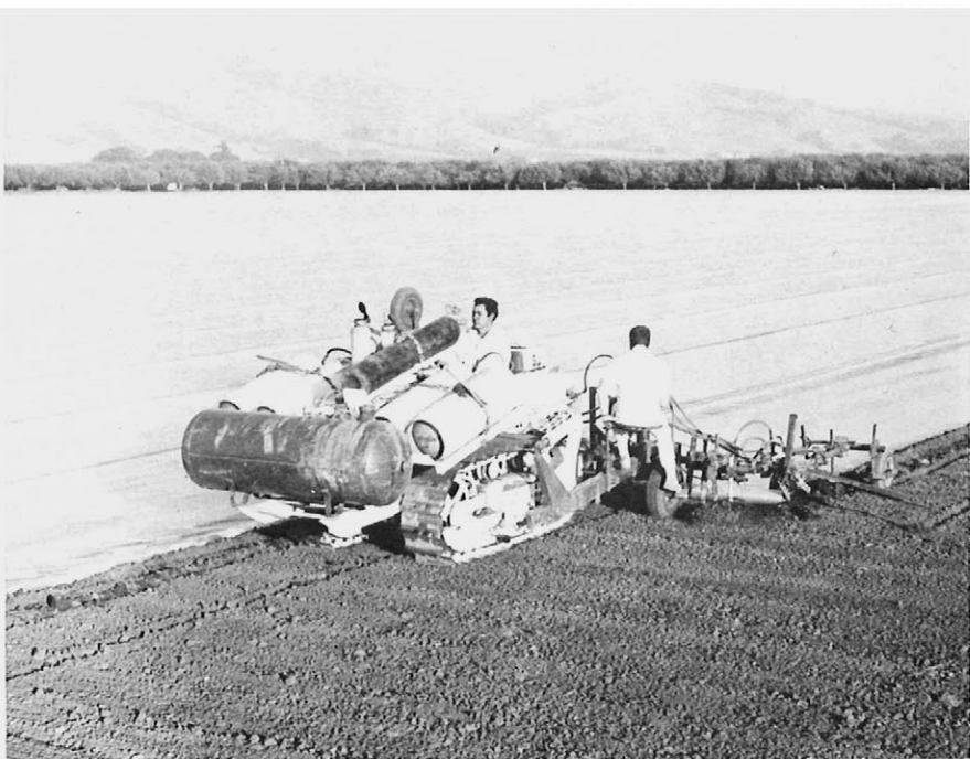
Fig. 2. Prospective strawberry land in California being fumigated with a mixture of methyl bromide and chloropicrin. Simultaneously with injection of fumigant, soil is covered with polyethylene film 0.025 mm (1 mil) thick. One edge of the film is glued to the preceding strip while the other is buried in the soil to provide resistance to wind. Soil remains covered for at least 48 hr. An experienced team can fumigate 25 acres in 1 day.
