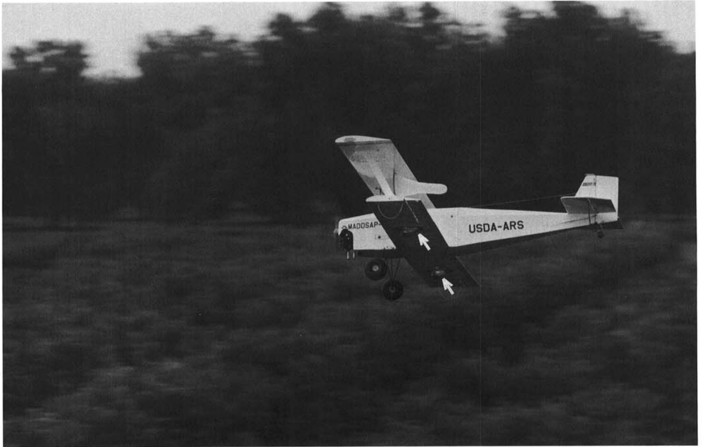
Fig 1. MADDAP-1 remotely piloted vehicle collecting spores and pollen approximately 15 m altitude above a peach orchard. The arrows show the positions of the pair of aerial spore/pollen traps.
