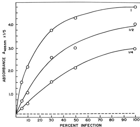
Fig. 7. Plots of enzyme-linked immunosorbent assay (ELISA) test absorbances against "percent infection", derived from plots of variation of absorbances with dilution (using healthy plant extract) for artificial mixtures containing 5, 10, 30, 50, and 100% extracts from 3-wk-old soybean mosaic virus-infected progeny plants mixed with extracts from healthy plants.
