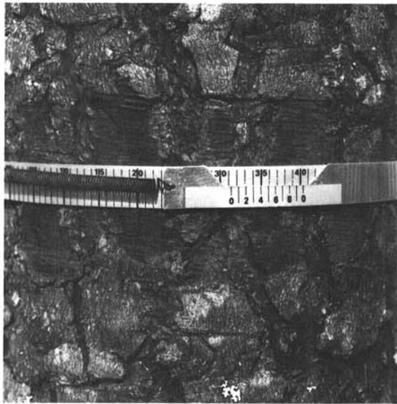
Fig. 1. Vernier scale dendrometer band in place on a stem of Pinus radiata . The spring which holds the aluminum band in place is attached again to the band, out of the picture, left. Tree growth expands the spring which changes the relative position of the scales and allows growth increments to be calculated. This scale reads (79.5 mm) 3.13 inches.
