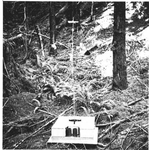
Fig. 1. Propeller anemometer and spore deposition sampler at Marckworth Forest. Two petri plates containing selective media were exposed at one time.
