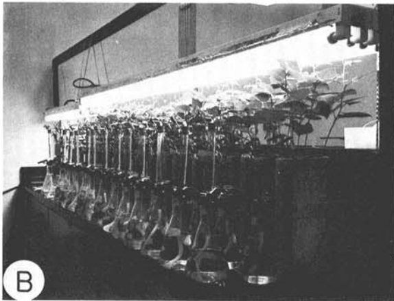
Fig. 1—(A, B). A) Diagram of apparatus used to evaluate effects of soil water matric potential, soil layer bulk density, and root rot infestation on growth of beans. Soil slab is clamped between the lucite and ceramic plates and water potential in the ceramic plate is controlled by regulated vacuum. B) The assembled units in use.
