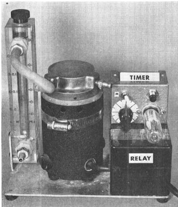
Fig. 1. New timer attached to K-C sampler relay case.
