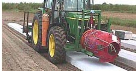
Fig. 30. Application of 1,3-dichloropropene after the beds are prepared using the Under Bed Fumigator, which limits worker exposure to the fumigant.
