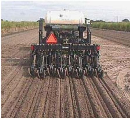
Fig. 21. Broadcast application of 1,3-dichloropropene using the Yetter deep placement coulters system.
