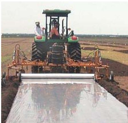
Fig. 17. Broadcast application of methyl bromide using 12 foot-wide polyethylene tarps.
