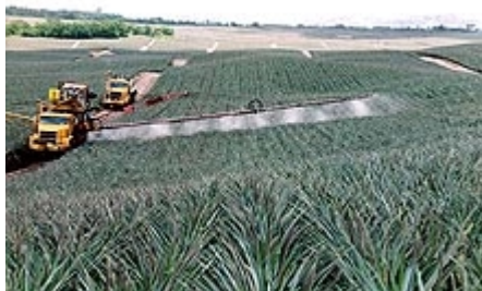
Fig. 5. Application of insecticide by means a long arm boom sprayer extending both sides of supplier truck. Insecticide is applied multiple times during the flowering season.
