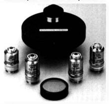
HMCS are: 1) the modulator, a special amplitude filter placed in the back focal plane of the objective; 2) a slit, partially covered by a polarizer, located at the
