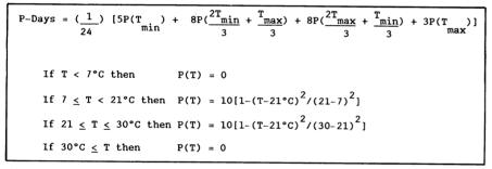
Fig. 1. Formula used for calculating the accumulation of P-Days for a 24-hr period. T = temperature,  $T_{min} =$  daily minimum temperature, and  $T_{max} =$  daily maximum temperature.
