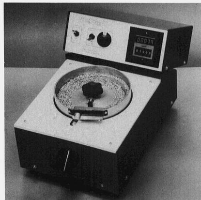
bowls for counting specific-diameter seeds (sizes available are 2.5, 4, 6, 8, and 10 mm) and a universal bowl that is adjustable from 1 to 10 mm. A BCD output is also available for use with a printer.
