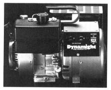
electric motor starting power is ¼ hp. The 44-lb generator features a USDA forestry approved muffler, automatic reset overload protection, automatic throttle control, a 76-cc 4-cycle engine, and two 120-V outlets.
