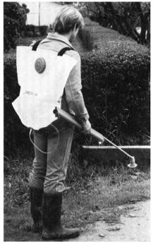
reservoir, which replaces the standard 2.5-L bottle, operates continuously up to 5.5 hr without refilling. The totally self-contained HERBI is battery-operated.
