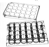
Each well in the distortion-free polystyrene plate is 16 mm in diameter and coded separately. The untreated lid reduces condensation, and special lid rings and raised well rims reduce cross-contamination of tissue cultures. Recessed areas between the wells also help reduce cross-contamination during filling procedures. Well bottoms are on the same plane for quick, accurate microscopic scanning.
