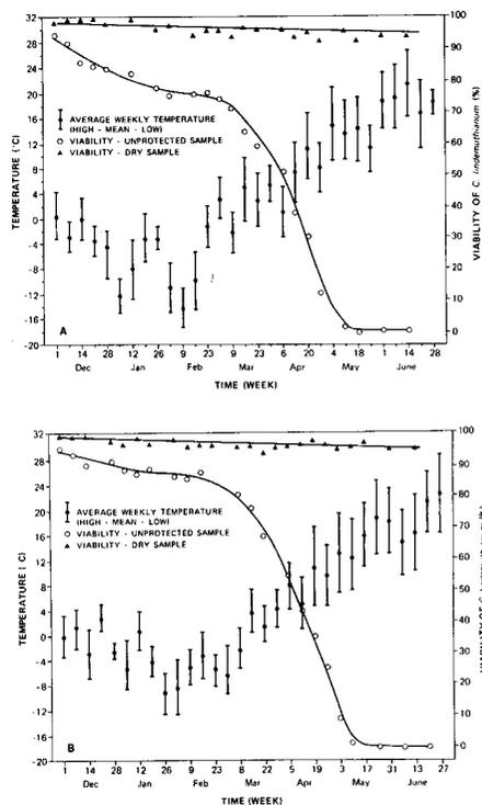
**Fig. 1.** Effect of field temperature on survival of *Colletotrichum lindemuthianum* on dry bean pod segments or seeds in a nylon-mesh pouch or in a waterproof polyethylene bag buried in the field (A) November 1978-June 1979 and (B) November 1979-June 1980.
