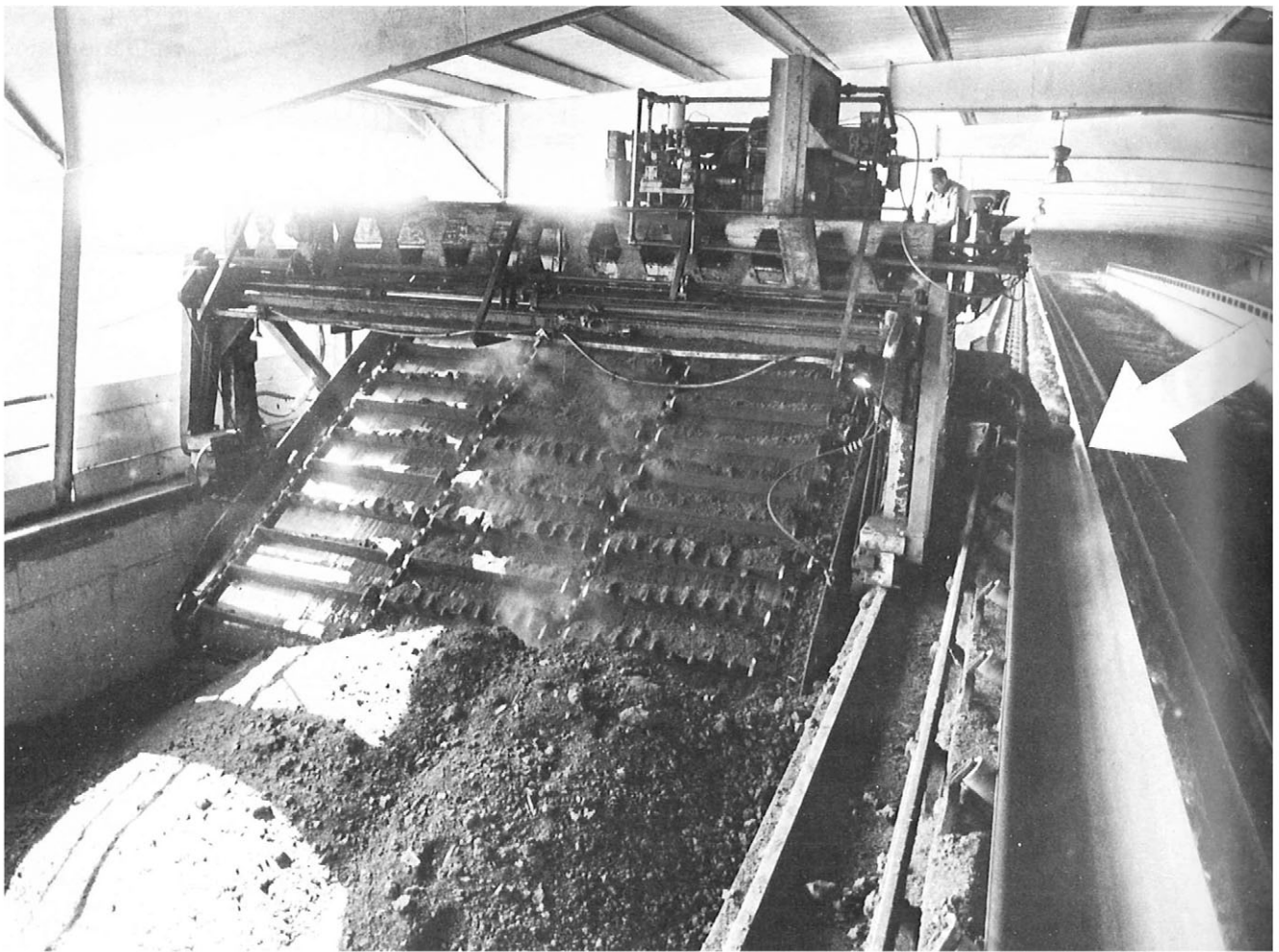
Fig. 1. Compost being removed from an aerated bioreactor tank and placed onto conveyor belt (arrow). The compost is aerated by fans through perforated floors and turned frequently to expose all organic matter to thermophilic conditions. Tank (4 × 7 × 150 m) on left is filled with cow manure and tank on right is filled with hardwood bark.
