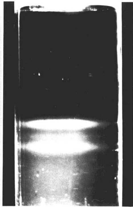
Fig. 3. Separation of nucleoprotein components of Prunus necrotic ringspot virus isolate FG by rate zonal centrifugation. Faint middle zone was visible. Preparation was centrifuged in 10–40% sucrose gradients in a Beckman SW 25.1 rotor at 24,000 rpm for 6 hr. Sucrose was dissolved in 20 mM phosphate buffer, pH 8.0.
